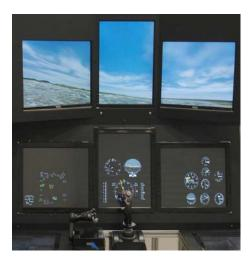
environment. The VCS is configured for close replication of a specific cockpit layout and switch/gauge logic. The VCS uses our MUSE<sup>™</sup> simulation software and can be configured to meet your specific training requirements.
