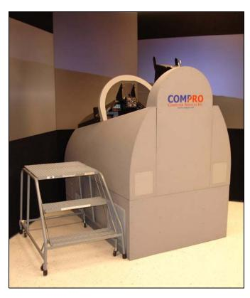
All functional controls, instrument panels, and cockpit hardware used are representative of the actual aircraft parts and reflect the same mechanical characteristics; that is, look, feel, and operate like the actual component. Non-functional components include silk-screened panels and components that are not connected to the I/O system.
