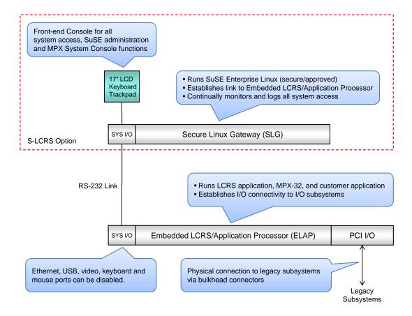
The ELAP executes a combination of customized kernel, LCRS application, legacy MPX-32 operating system, and legacy binary application code. Because of the custom kernel, the ELAP is truly an "embedded" solution.
